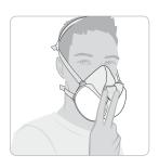
Close the vents of the exhalation valve by pressing down the flexible valve cover and breathe out slowly. If no air escapes between facepiece and face, a proper sealing fit is achieved. If air escapes, adjust the position of the mask on the face or adjust the tension of the straps. Repeat this check until a seal is achieved. If a secure seal cannot be achieved, do not enter any contaminated area. See your supervisor.
